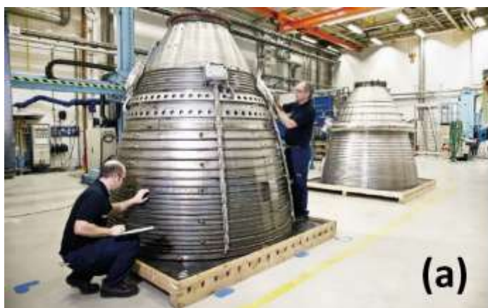
Figure 7(a) More than 50 kg of DED material was used as the demonstration nozzle for the Vulcain 2 [222]; (b) AW350 XWB AM Titanium Brackets [223].
