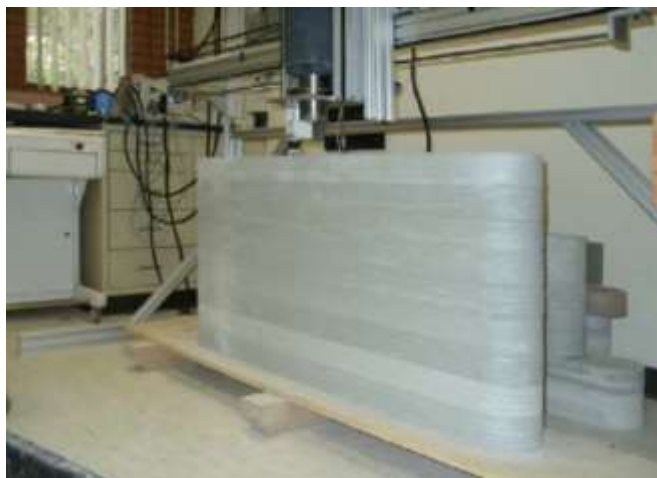
Figure 5: Concrete building that was 3D printed (courtesy of Zareiyan and Khoshnevis [148]).
