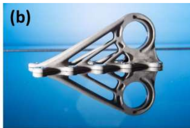
Figure 7(a) More than 50 kg of DED material was used as the demonstration nozzle for the Vulcain 2 [222]; (b) AW350 XWB AM Titanium Brackets [223].
