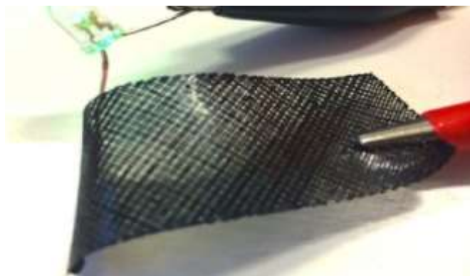
Figure 3: The first 3D-printed nanocomposite made of multi-walled carbon nanotubes (courtesy of Postiglione et al. [91]).
